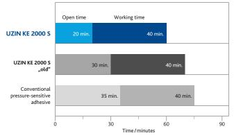
PVC sheet installation on UZIN NC 170 LevelStar, notch size A 2, at 20  $^{\circ}\mathrm{C}$  and 65 % relative humidity.
